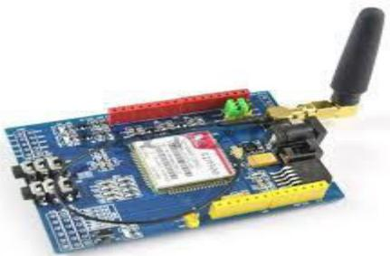
**Fig 3:** GSM Module
